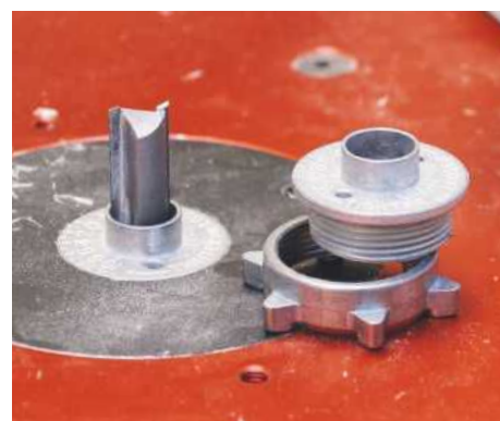
▲ The jig comes with the 2-part eBush
